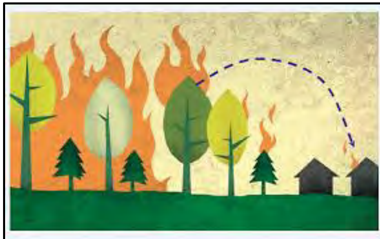
Figure 3. Illustration of spotting during a wildfire (Adopted from http://www.firewise.org ). Spotting occurs when embers from burning material gets transported by the wind which has the potential to start new secondary fires.
